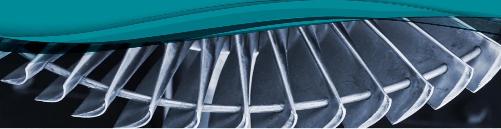
The UK arm of a global manufacturing company specialises in the manufacture of impellers for automotive turbochargers and aerospace turbojet engines. Fully automated 5-axis machining of the titanium, Inconel and forged aluminium impellers requires high precision and very predictable tool wear. The manufacturer runs 32 machines on site, both roughing and finishing the impellers.
