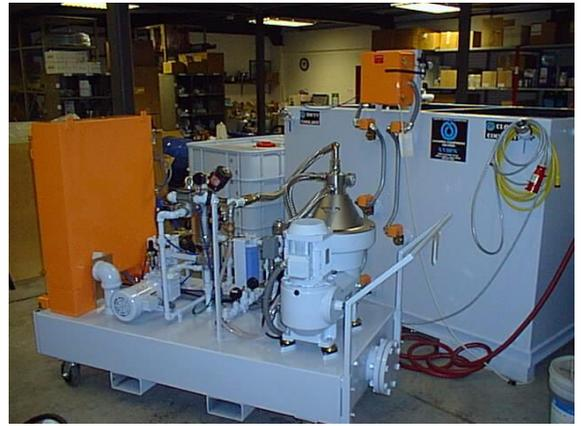
The unit is equipped for use on high temperature and high pH fluids. And being mobile, it is able to process fluids in different locations within the Sunderland factory. With a flow rate of 750-1400 litres per hour dependant on the type of fluid used, the XYBEX® removes both free and emulsified tramp oil to 0.5% or less and particles down to 8 micron or less.
