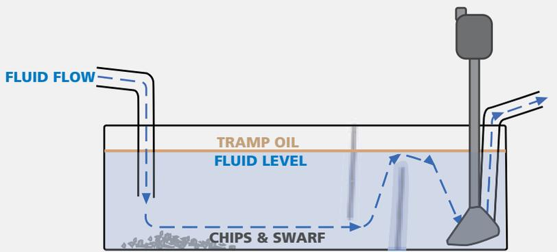
**ILLUSTRATION OF TANK WITH COOLANT SUMP**
