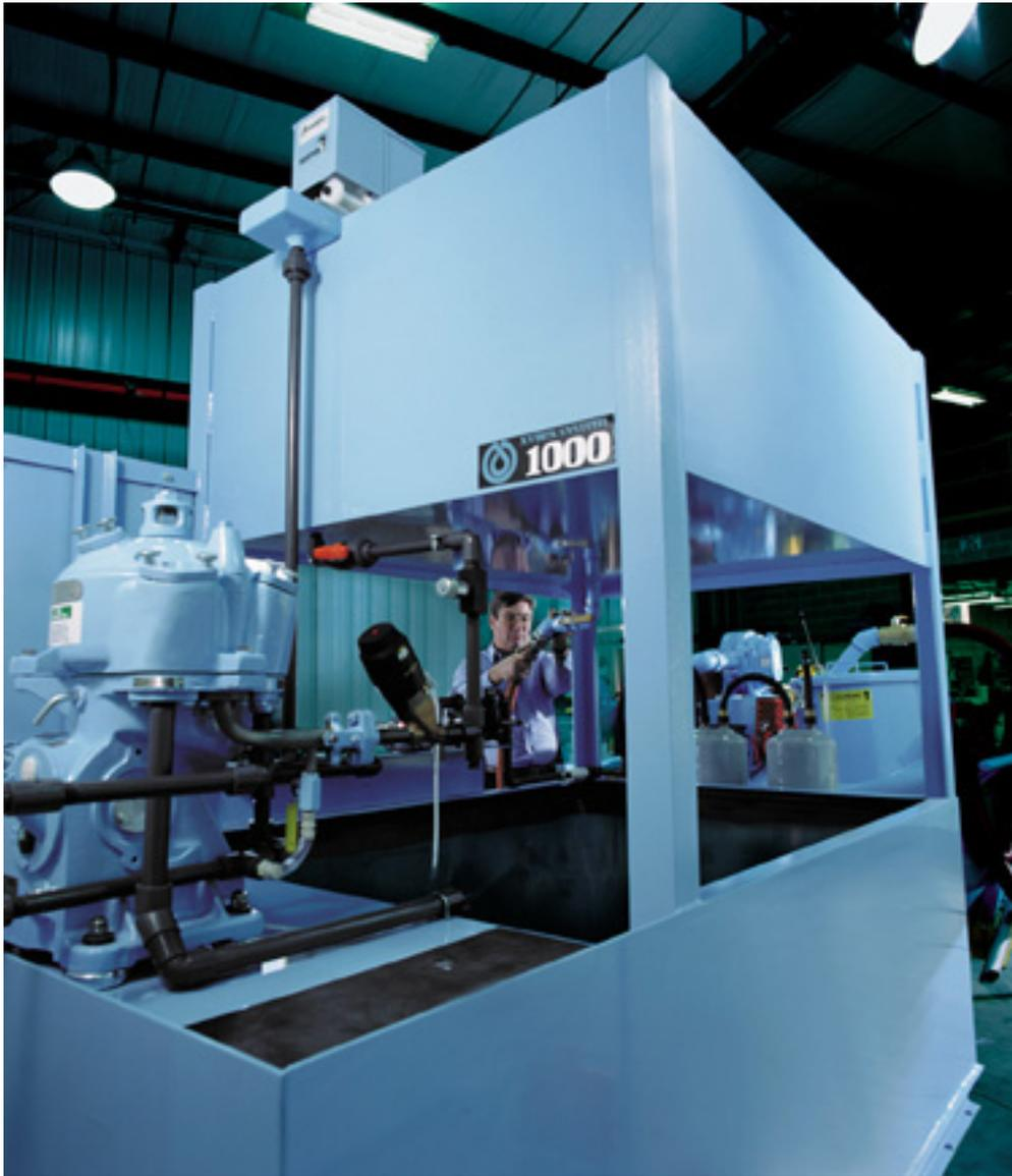
***Figure 2. Dirty fluid (collected with a yellow-bellied sump sucker) is pumped into a XYBEX 1000 coolant recycling system.***
