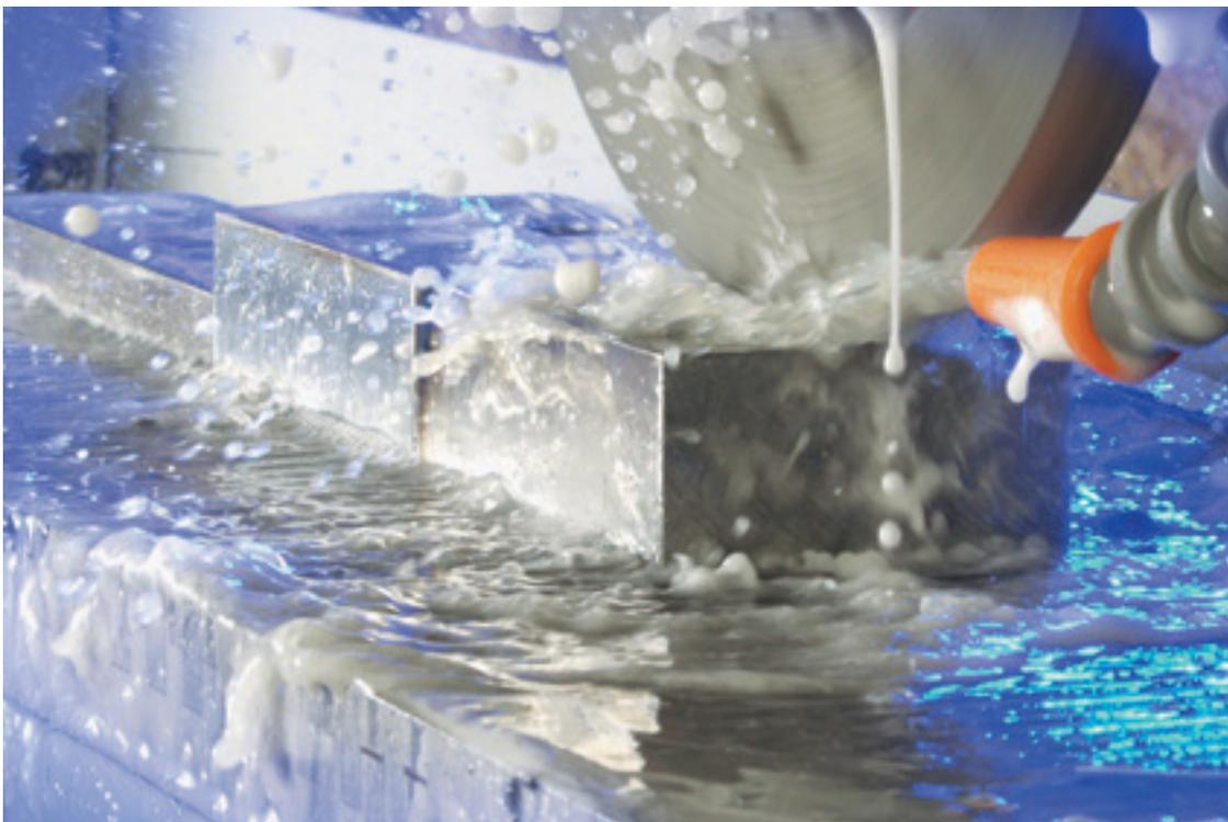
***Figure 3. A TRIM® C320 being used to surface grind. Coolant management is especially important in grinding, where the fluid is quickly contaminated with the grinding swarf.***
