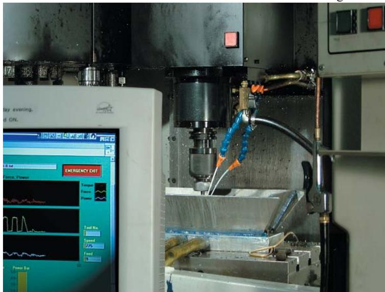
*Testing the forces on the metal during a drilling operation.*
