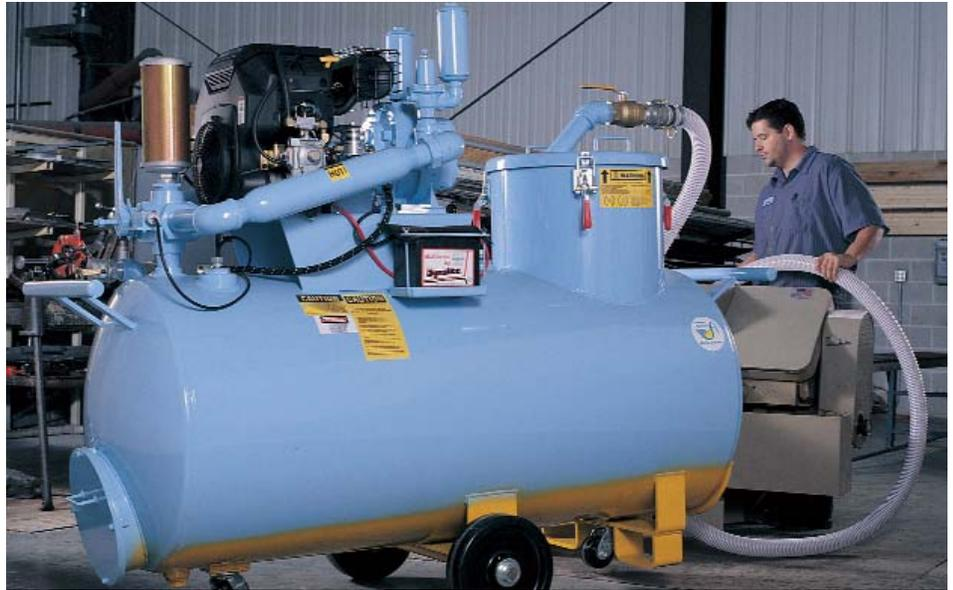
*Cleaning out a coolant sump with an LP Gas Yellow Bellied Sump Sucker from the Master Chemical Corporation*
