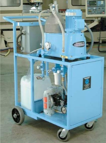
*The Tramp Oil Terminator from the Systems Equipment Division of Master Chemical is a robust centrifuge unit, generating 6,500 Gs of centrifugal force, processing as much as two and one-half gallons of coolant a minute, depending on the type of coolant used and its condition.*
