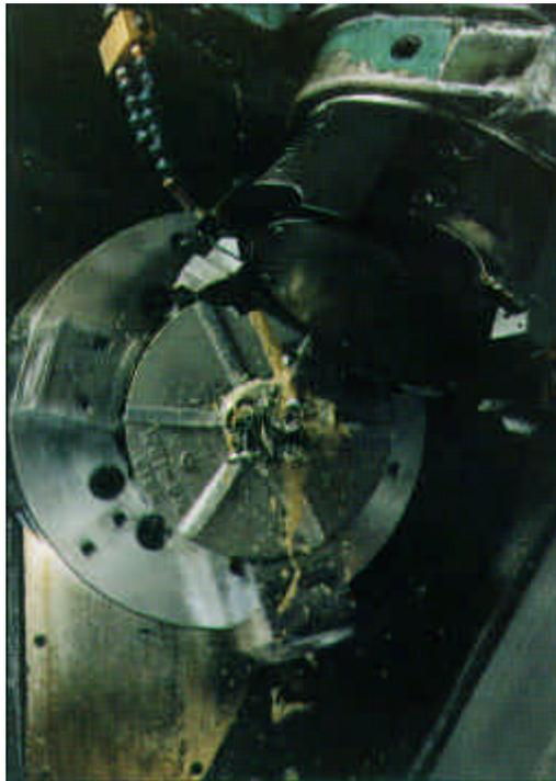
**Nonchlorinated cooling and lubricating fluid is being used in turning stainless steel pump impellers on a Cincinnati Milacron Cinturn at Aurora/Hydramatic Pump, Ashland, OH. TRIM® SC 210 is free of chlorine and sulfur EP additives, phenols, and nitrates, is easily recycled, has a long sump life, and rejects tramp oil.**
