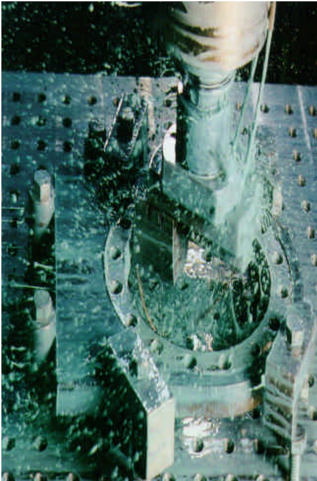
Lubrication reduces tool wear because cutting forces are decreased as friction at the face and flank of the cutting tool or abrasive grain is reduced. Lubrication also increases shear angles and, thereby, reduces work hardening and workpiece distortion ahead of the tools.
