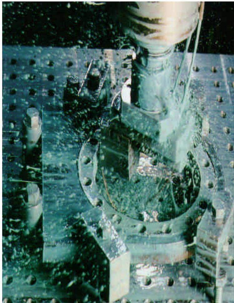
Cutting and grinding fluids provide lubricating and cooling effects which are absolutely essential to the economical production of precisely machined and ground parts. These precision parts, produced at high rates and low unit cost, are absolutely critical to the reliable, high-technology lifestyle we take for granted.
