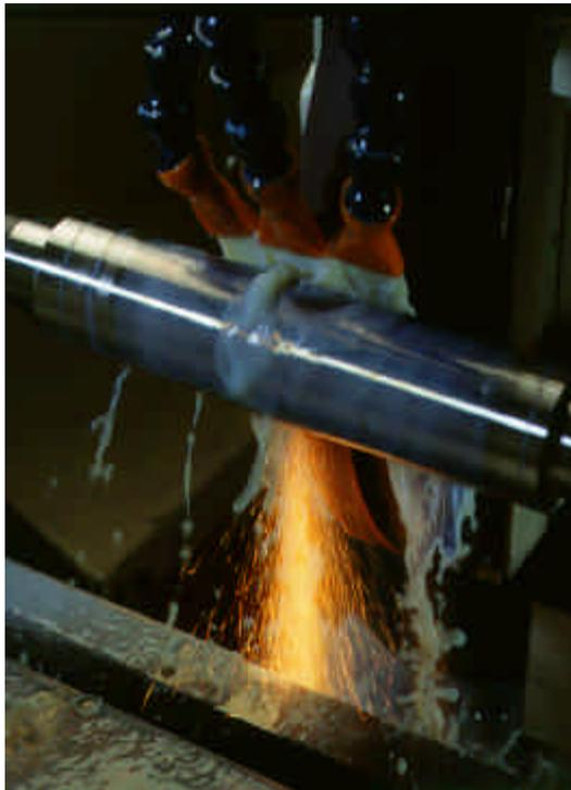
**King Machine Tool, Massillon, OH, finish grinds 4340 steel with 0.002” depth of cut using TRIM® E 190, a water-soluble, nonchlorinated fluid that can be recycled easily, and Radiac 80J 1” wheel, 24” in diameter.**
